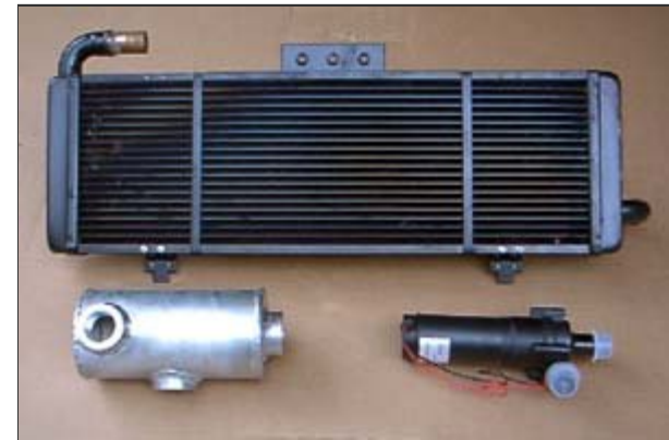
Intercooler radiator, coolant pump and filler tank
