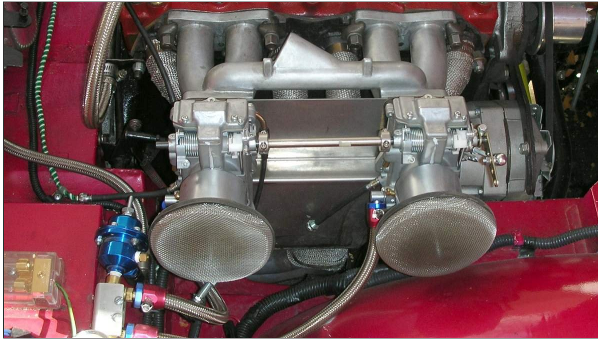
Mikuni air horns with screen filters on Jim Grey's TR4 vintage racer
