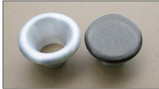
Mikuni air horns with screen filters on Jim Grey's TR4 vintage racer
